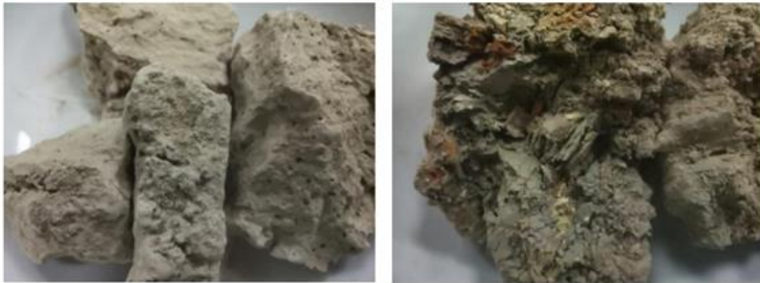
Fig. 1: Appearance of loam and bentonite clay deposits of the Turkestan region: a) loam; b) bentonite clay
