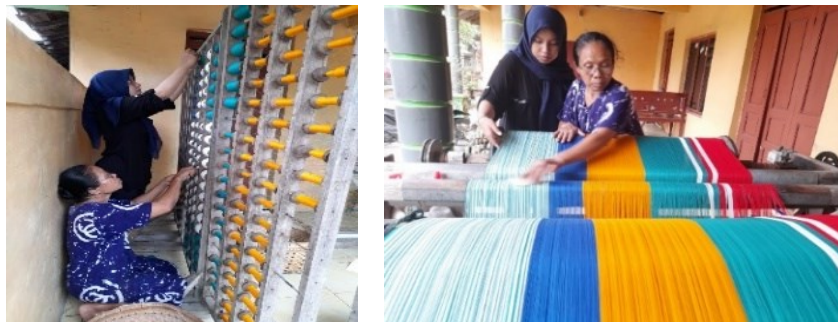
Fig. 3: The process of warping, configuring the order of the warp threads on the boom according to the design
