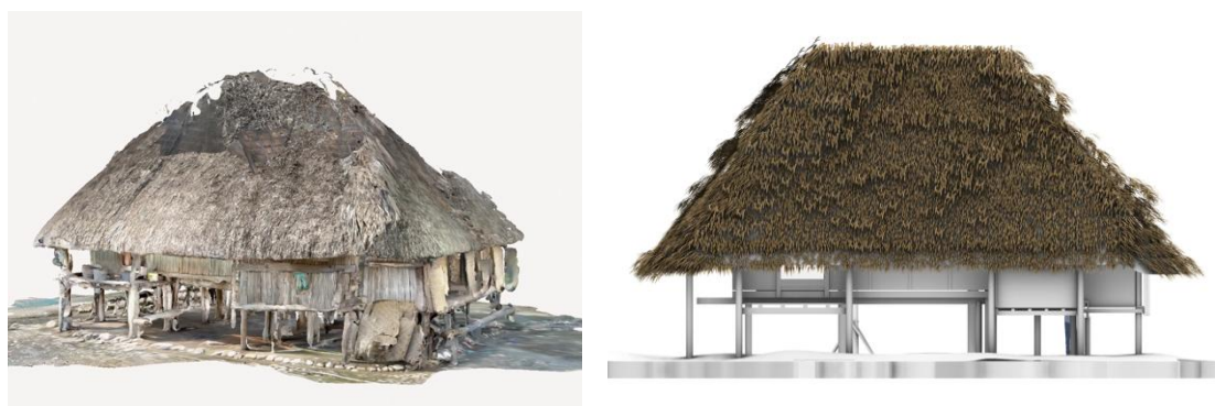
Fig. 3: Comparison of the raw LiDAR scan captured on site using Polycam Pro (left) and the refined model created after processing and alignment with photogrammetric data (right).
